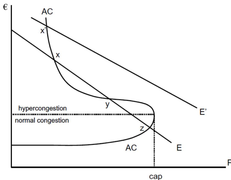
Figure 2. The backward-bending average cost curve (AC) and two inverse demand curves (E and E0) defined over traffic flow (F) (source: Verhoef, 2005)
