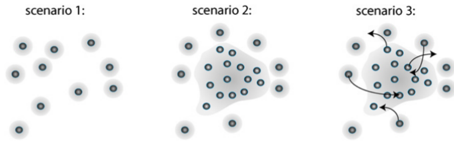
Figure 1.5: Schematic of droplet micro-mixing [30].
