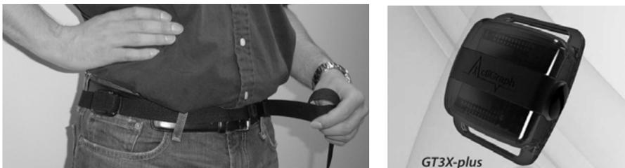
Figure 4.3: Actigraph GT3X-Plus accelerometer
