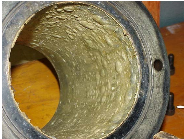
Figure 3.6 The failure of epoxy paint as cell's coating
