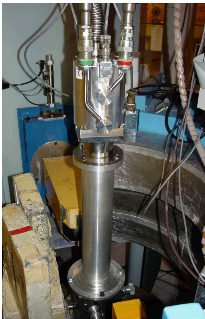
Figure 2.6: Photograph of the cryofurnace attachment in operation on the High Resolution Powder Diffractometer at HIFAR [12] .
