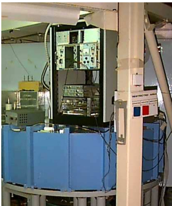
Figure 2.5: Photograph of the High Resolution Powder Diffractometer at HIFAR, Lucas Heights showing the blue coloured detector bank [10] .
