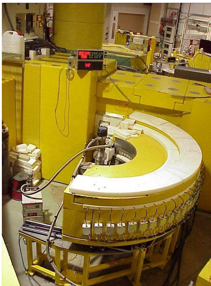
Figure 2.8: Picture of the BT-1 High Resolution Neutron Powder Diffractometer [15] .
